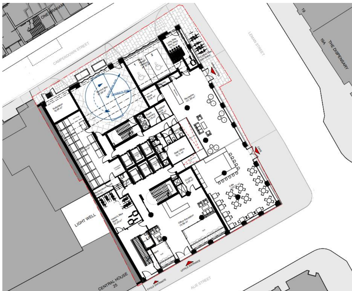
Figure 3: Ground floor arrangement of the proposed development showing the Aparthotel reception and café (right), office entrance (bottom) and servicing (top)
